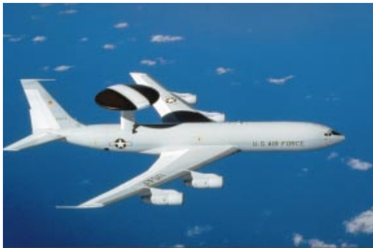
The E-3 is used for air and maritime radar surveillance, detection, and monitoring of suspected smuggler aircraft and vessels.
